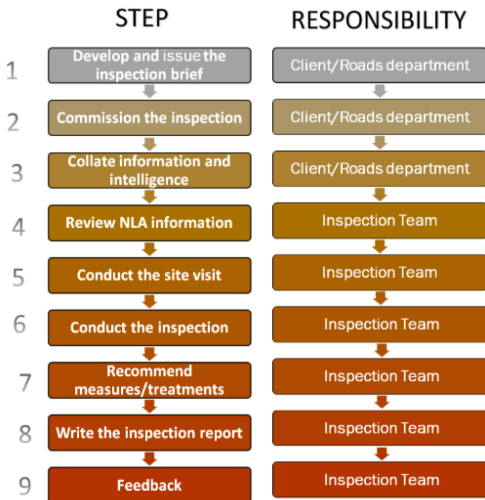
Figure 4-2: Inspection process flow chart
